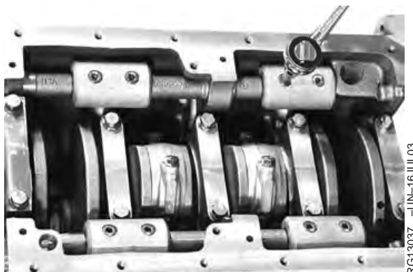
Remove Balancer Weights
