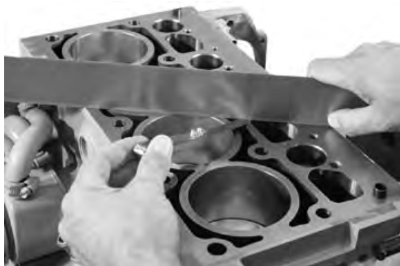
Measuring Cylinder Block Top Deck Flatness
