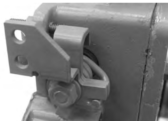
High Idle Lever Position
