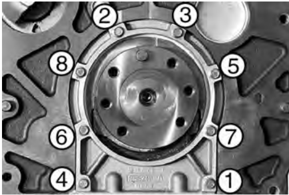
Rear Oil Seal Torque Sequence
