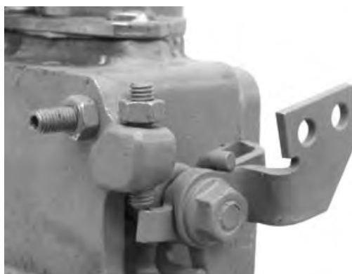
Low Idle Lever Position
