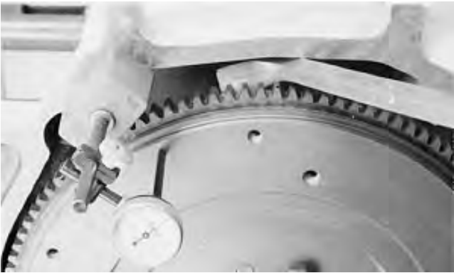
Check Crankshaft End Play w/Dial Indicator
