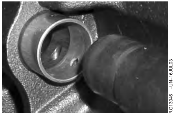
Align Oil Supply Holes
