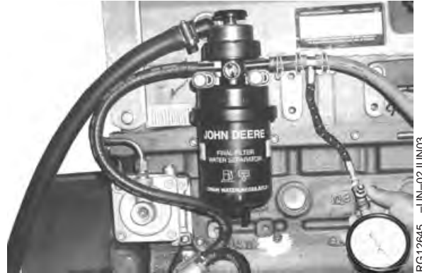
Supply Pump Pressure
