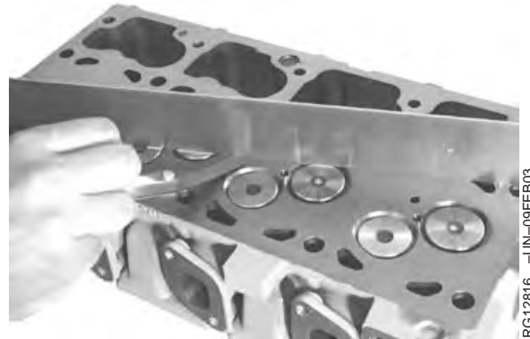
Cylinder Head Flatness Check
