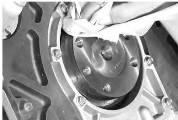
Clean Crankshaft Flange
