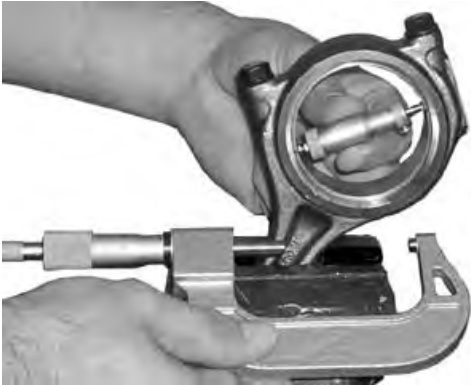
Measuring Rod Bearing ID
