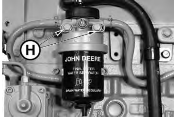
Remove Fuel Filter
