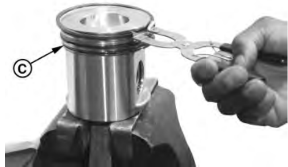
Piston Ring Expander Tool
