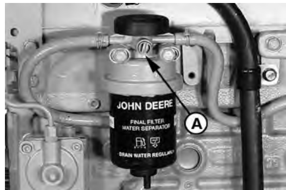
Fuel Filter Bleed Vent Screw
