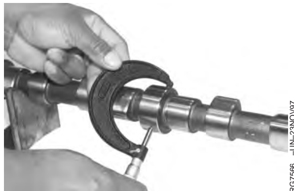
Measuring Camshaft Journal OD
