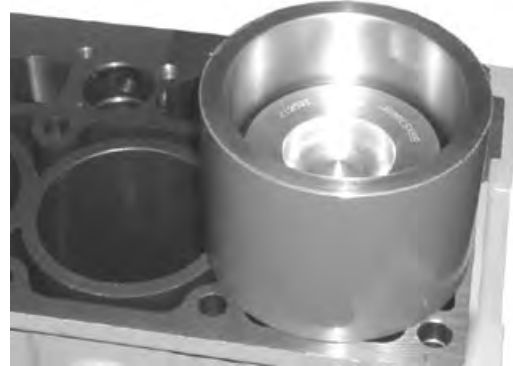
Install Piston—Tapered Ring Compressor
