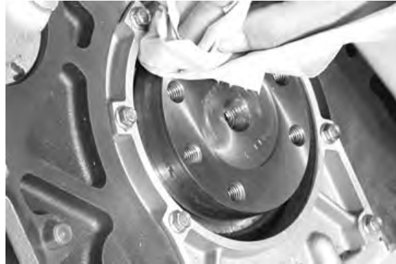
Clean Crankshaft Flange
