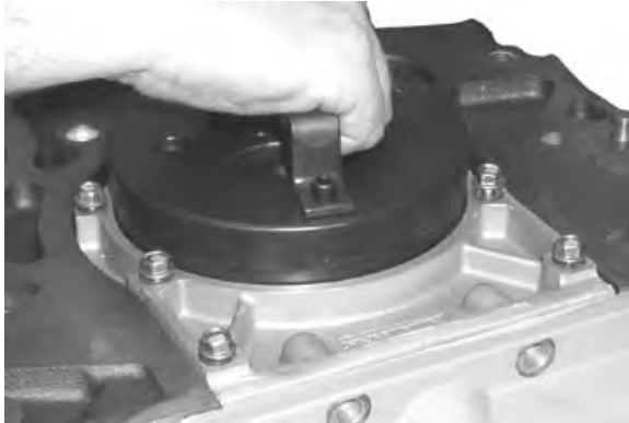
Rear Oil Seal Housing Aligner
