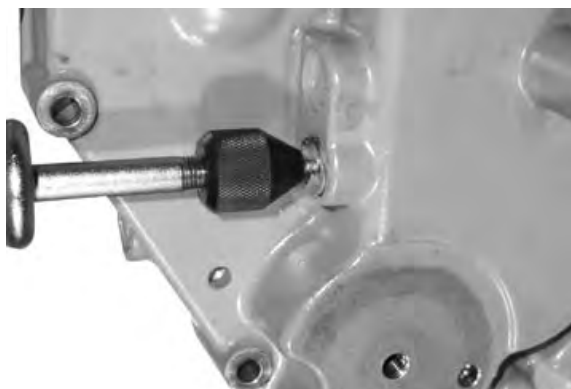
Remove Governor Shaft Cup Plug
