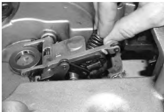
Remove Idle Bias Spring
